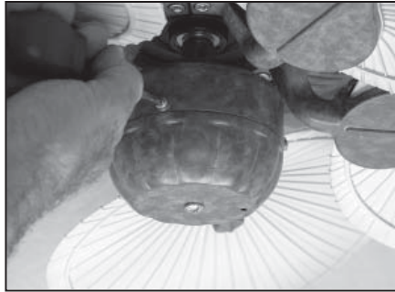
2. Remove cover switch housing.
