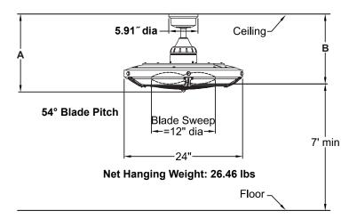
Fan must be attached to a securely anchored electrical junction box capable of withstanding a load of at least 35 lbs.
